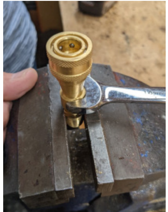
Figure 2: QD Removal Process - Unthread QD from Fitting.
