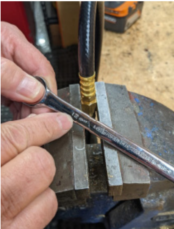
Figure 3: Plug Removal Process – Use 12mm Wrench.
