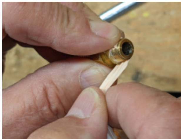
Figure 5: Plug Reinstall – Use Loctite or thread tape to install new QD's Wrench.
