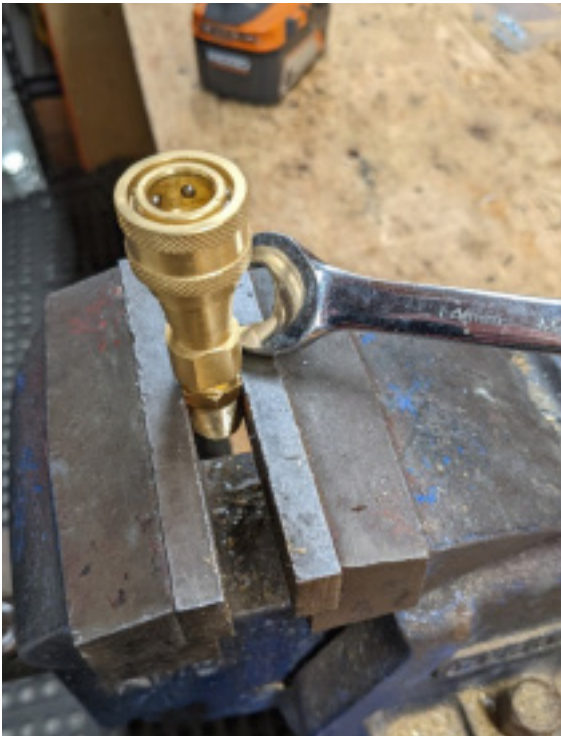
Figure 1: QD Removal Process - Use 14mm Wrench.
